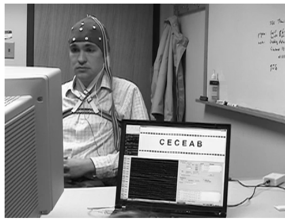
Figure 6: EEG-based recognition system for unspoken speech (Wester and Schultz (2006))
