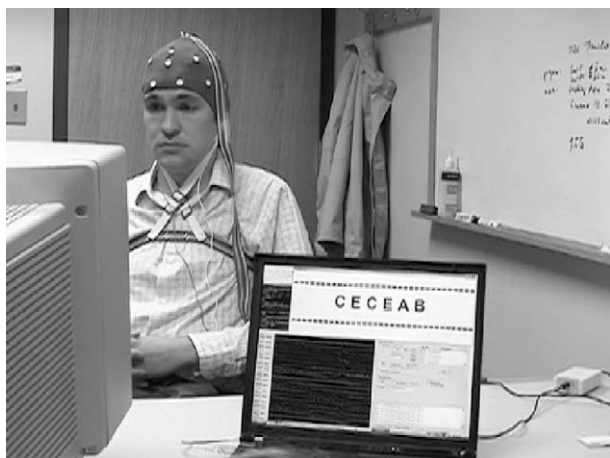
Fig. 6. EEG-based recognition system for unspoken speech (Wester and Schultz, 2006).
