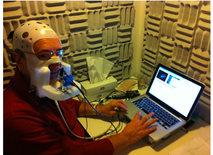
Figure 1. Speaker in sound cabin with form-fitted plastic acquisition helmet. Ultrasound probe is on white cable entering from below, lip camera is small blue box in front of mouth. Terason T3000 ultrasound machine is on small tray beneath portable PC running Ultraspeech.
