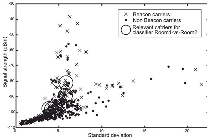
Figure 2. Signal strength and standard deviation of 500 available carriers scanned in room 1.
