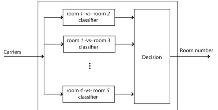
Figure 1. Overview of the system: the input “carriers” of the classifier can be all available carriers, “All”; or a subset thereof, “Standard” or “Relevant”.
